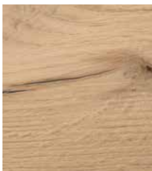
Rovere, con spaccature, G5 Oak, fissured, G5
